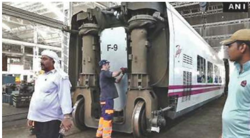
A coach being inspected. The articulation is clearly visible
