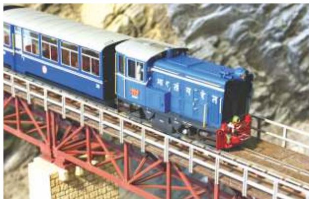
The Darjeeling NDM6 is made from a British Backwoods Models brass kit for the body and a scratch built chassis. The coaches are Worsley Works' kits
