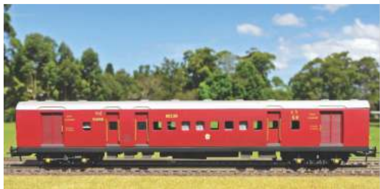
Here is a model of an SLR made from a Shinkansen coach, which is fairly accurate, aside from the visible underframe, which does not exist on the integral bodied coaches built by Indian Railways
