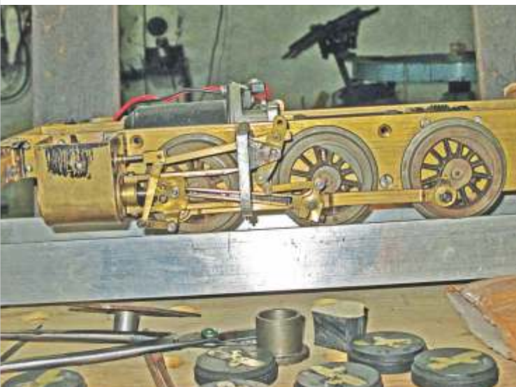
Under gear of locomotive model "Indian Glory"
