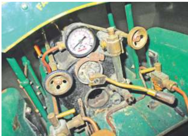
Pressure gauge and throttle of the Fairy Queen
