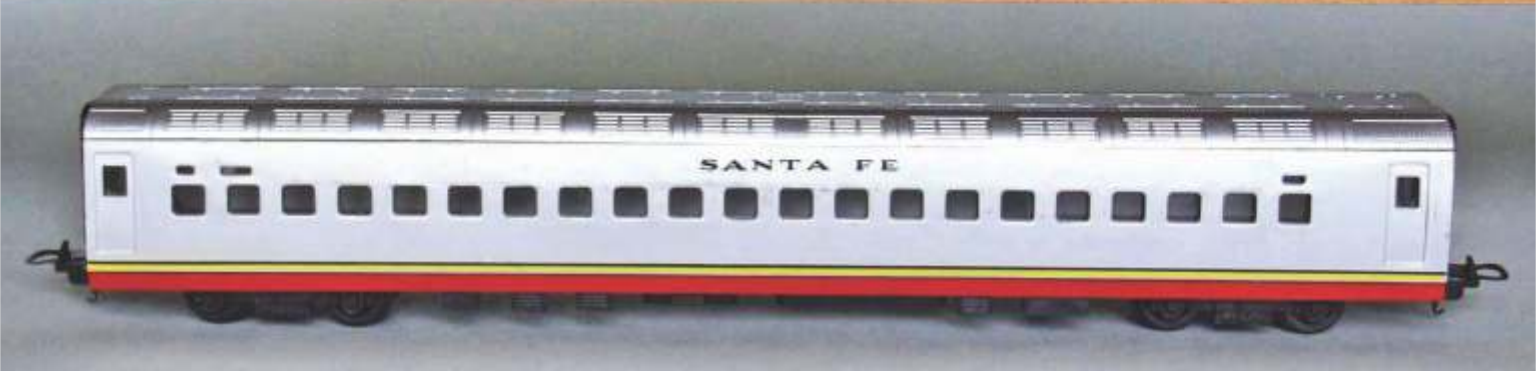
Cheap models of the Japanese Shinkansen coaches provide the basis for quite accurate models of many Indian coaches. The Shinkansen coach shown was marketed in a fictitious 'Santa Fe' livery, as a toy for the US market
