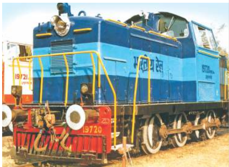
A diesel-hydraulic WDS4B class loco, fitted with Suri transmission
