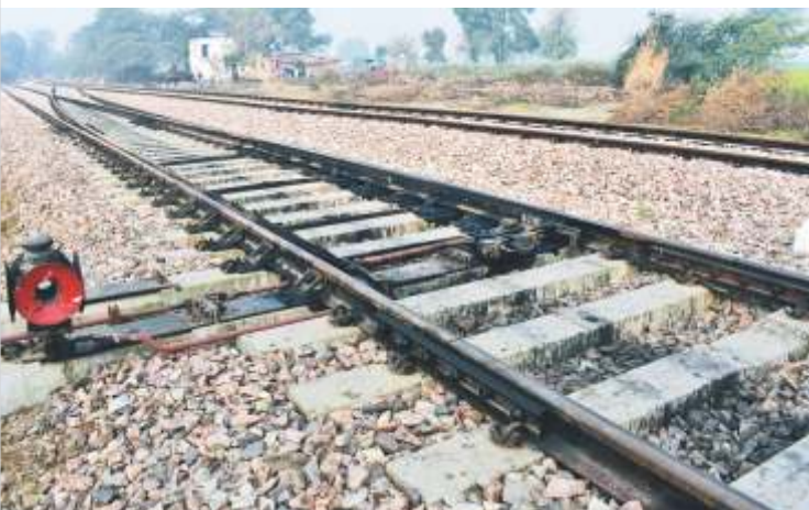
Shunting signal with manual inter-locking
