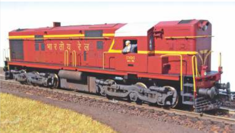
This WDM2 was modified from an Australian class 45, which is a similar ALCO design. The main changes were adding cowcatchers and shifting the cab closer to the end
