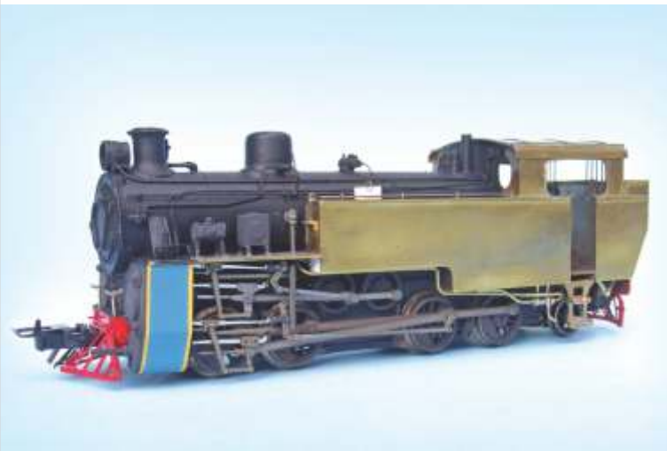
The HO model of a Nilgiri X class 0-8-2 rack loco. This was scratch built, apart from the wheels, motor and some of the valve gear. At this stage the body had not been fully painted
