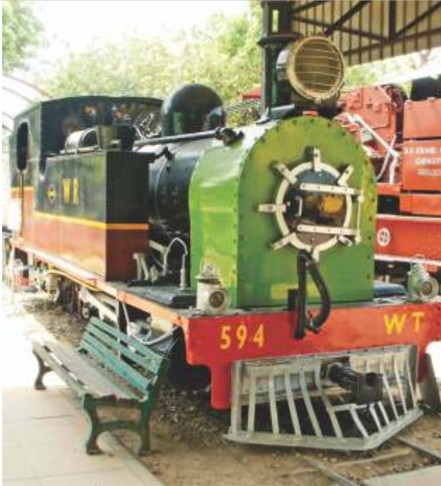
WT 594, a 0-6-4 NG loco imported from W.G. Bagnall in 1926
