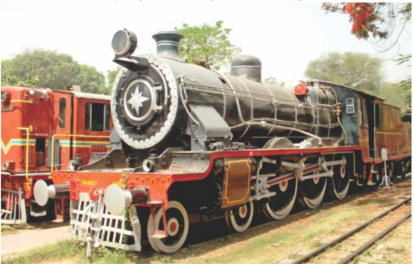
Loco No. 24467 HPS-2 a 4-4-0 loco imported by the East Indian Railway in 1950 from Vulcan Foundry Limited
