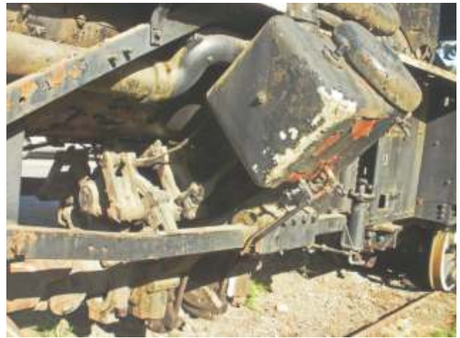
One of the cylinders of the Heisler loco
