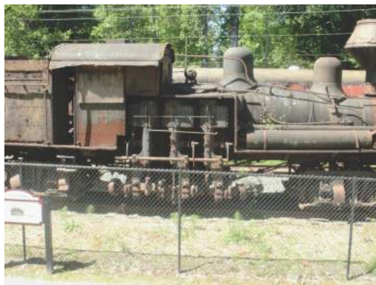
The 3 vertically placed cylinders of the Shay
