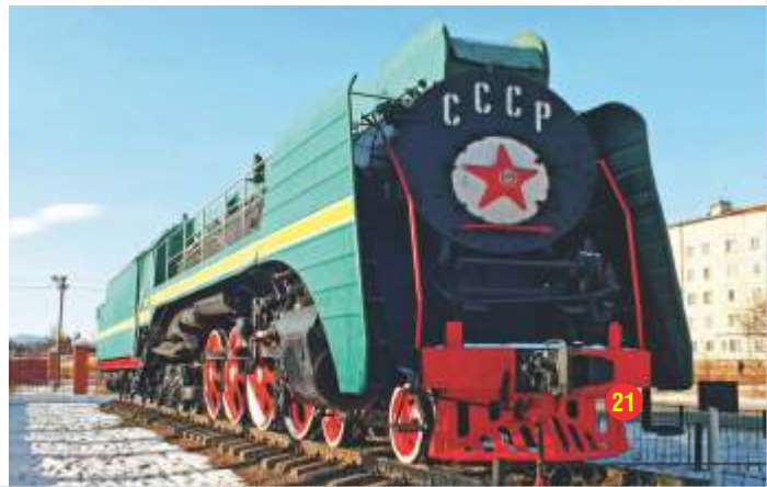
Severobaikalsk. Plinthed P36 Class 4-8-4. 251 were built between 1950-1956, the last express passenger loco type built for Soviet Railways
