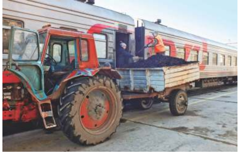
▲ Steam Lives On—But only for the coal-fired heating boiler in each carriage!
