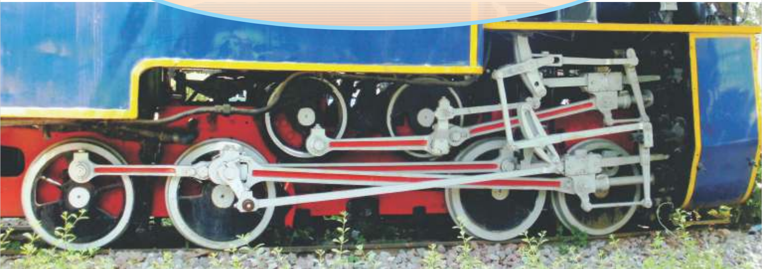
Eccentrics and cranks of a steam locomotive
