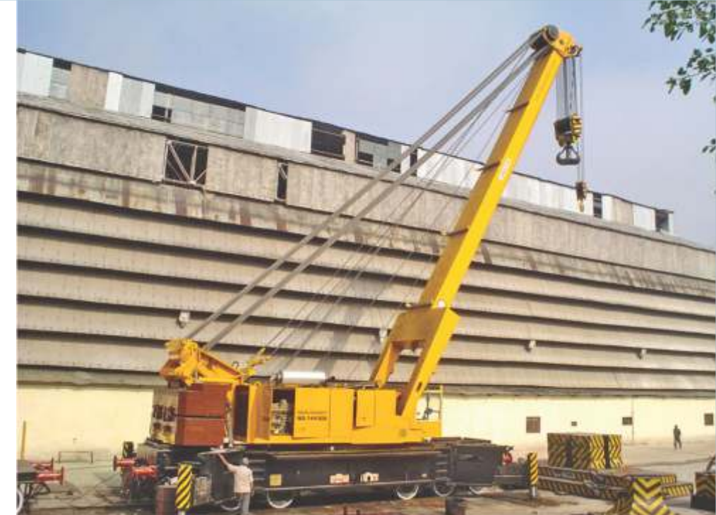
One of the rail-mounted breakdown cranes used by the railways for track clearance following an accident. This crane has a capacity to lift 140 Tonnes and is manufactured at the Railway Workshop at Jamalpur
