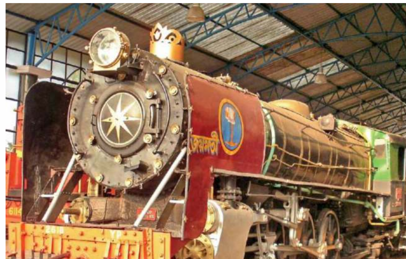
A Tata Engineering & Locomotive Company Meter Gauge YP class locomotive, built in 1970. It is now exhibited at the Heritage Park, Tinsukhia. This and the photograph below appear in Vikas Singh's book
