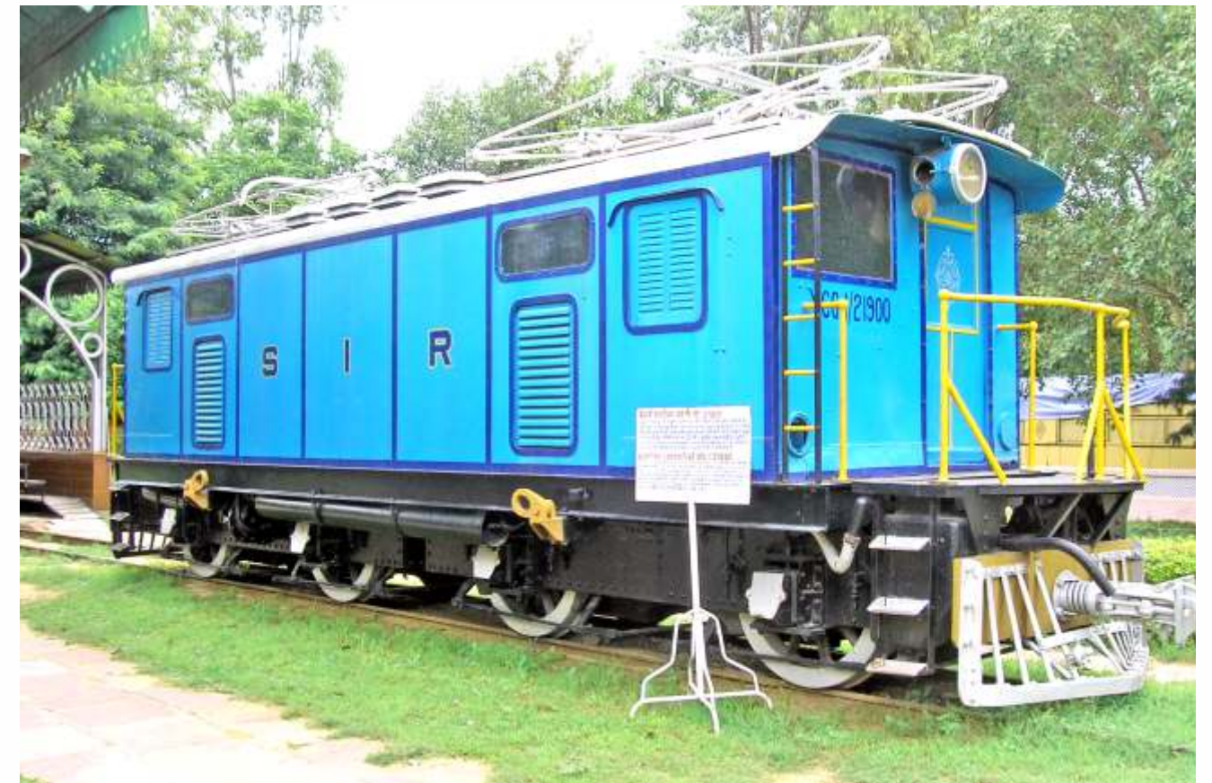
A YCG1 locomotive. This worked around Chennai area, the only part of the Indian Railways Meter Gauge network that was electrified Kalyan, near Mumbai, was one of the few sheds that homed dual-voltage locomotive that could work on AC as well as DC. This is a WCAM3
