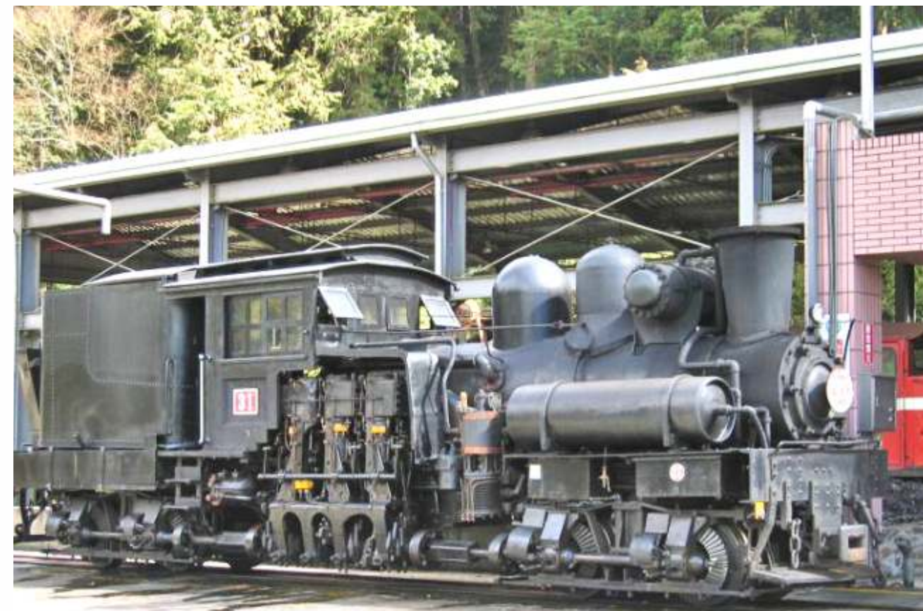
A 'Shay' geared steam locomotive that is in use on the Alishan Forest Railway
