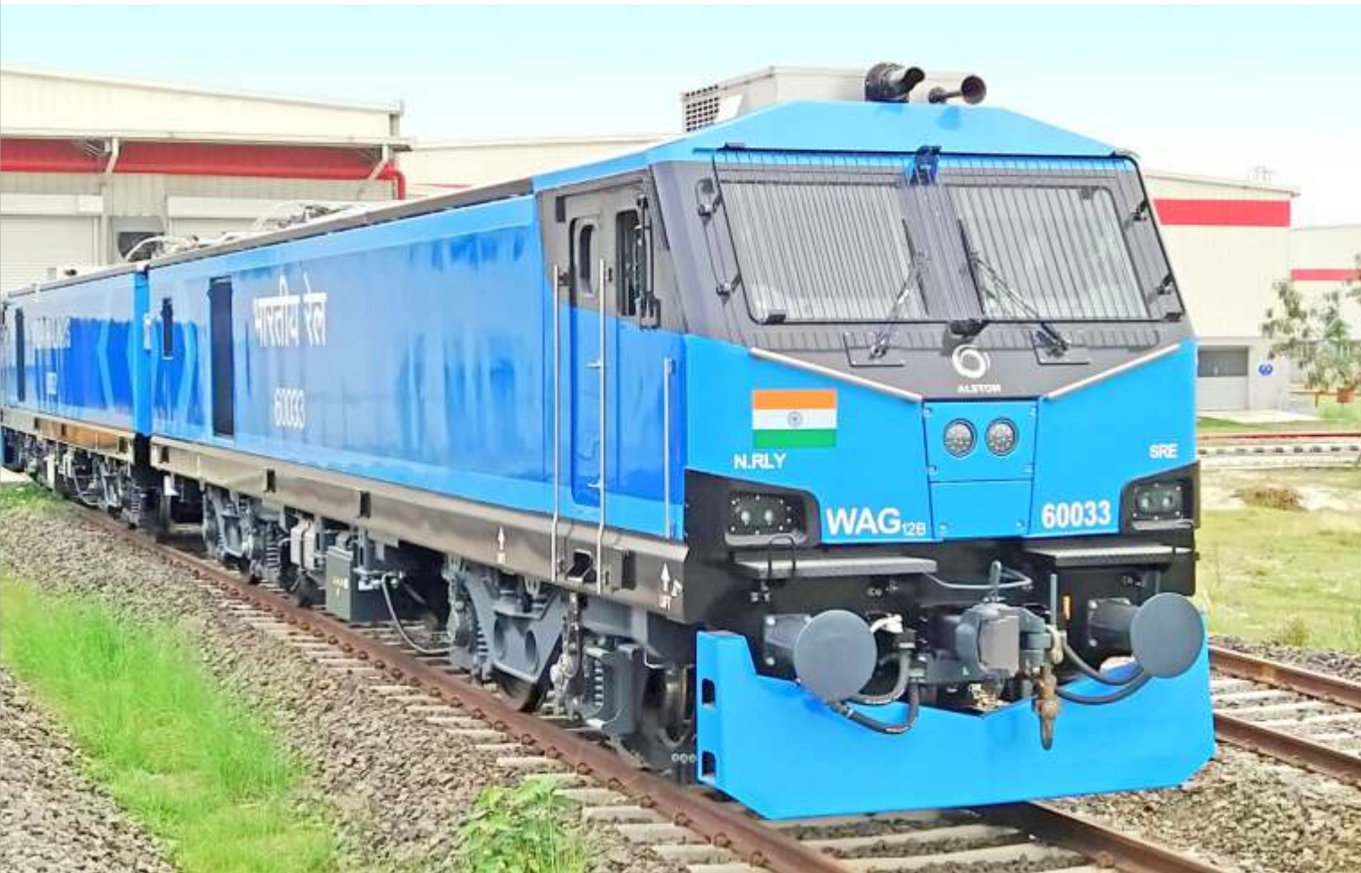
The most powerful locomotive in the country: a 12000 HP WAG12. The loco has two units permanently coupled
