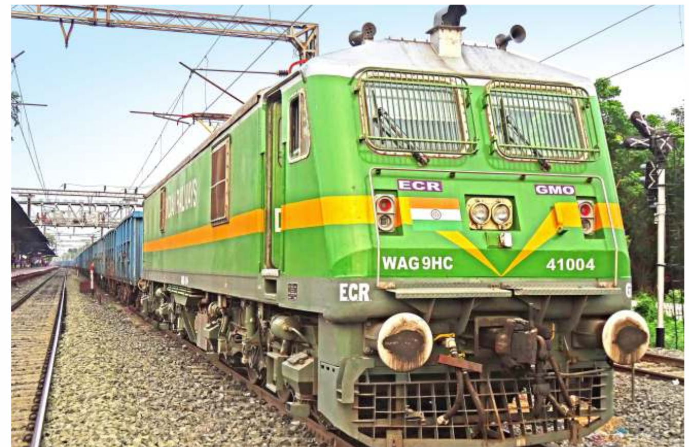
A WAG9HC class locomotive. Generating 9000 HP, this is the most powerful single unit loco in the country. Only the double unit WAG12 is more powerful A passenger train hauling locomotive, the WAP5
