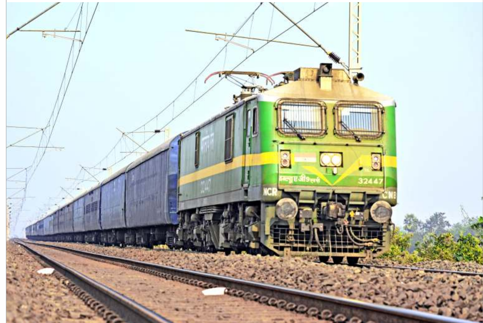
The freight locomotive, the WAG9 class which was modified to create the WAP7
