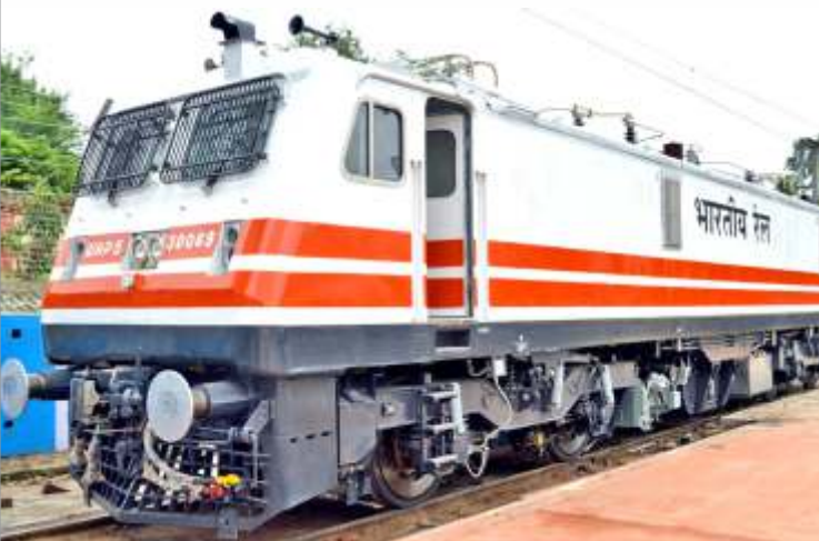
A WAP-5 class locomotive. CLW is working to use these locos in push-pull mode (Cont'd from Page 29)
