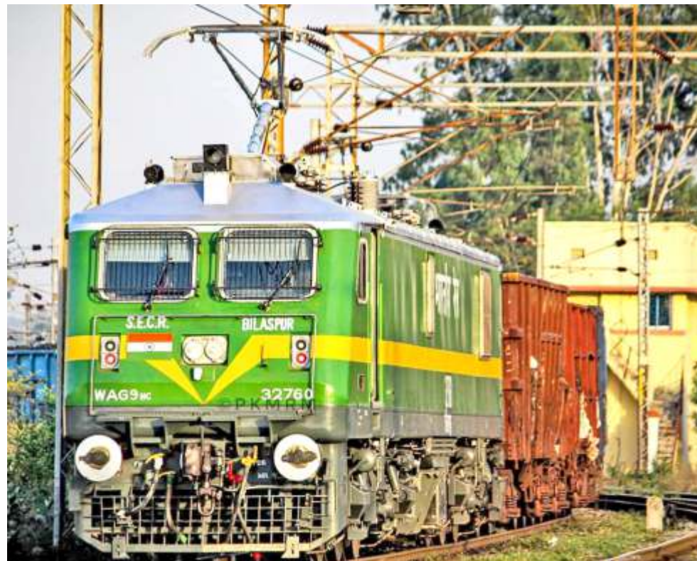
A WAG-9 class locomotive. CLW adopted 3-phase technology on this class
