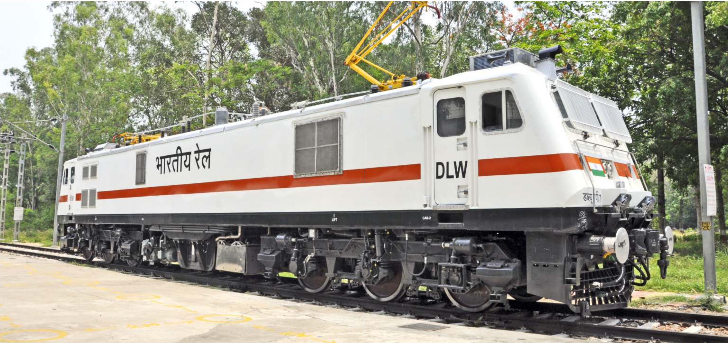
A WAP7 class locomotive manufactured at DLW. Earlier manufacturing diesel locomotives, DLW now turns out electric locos only
