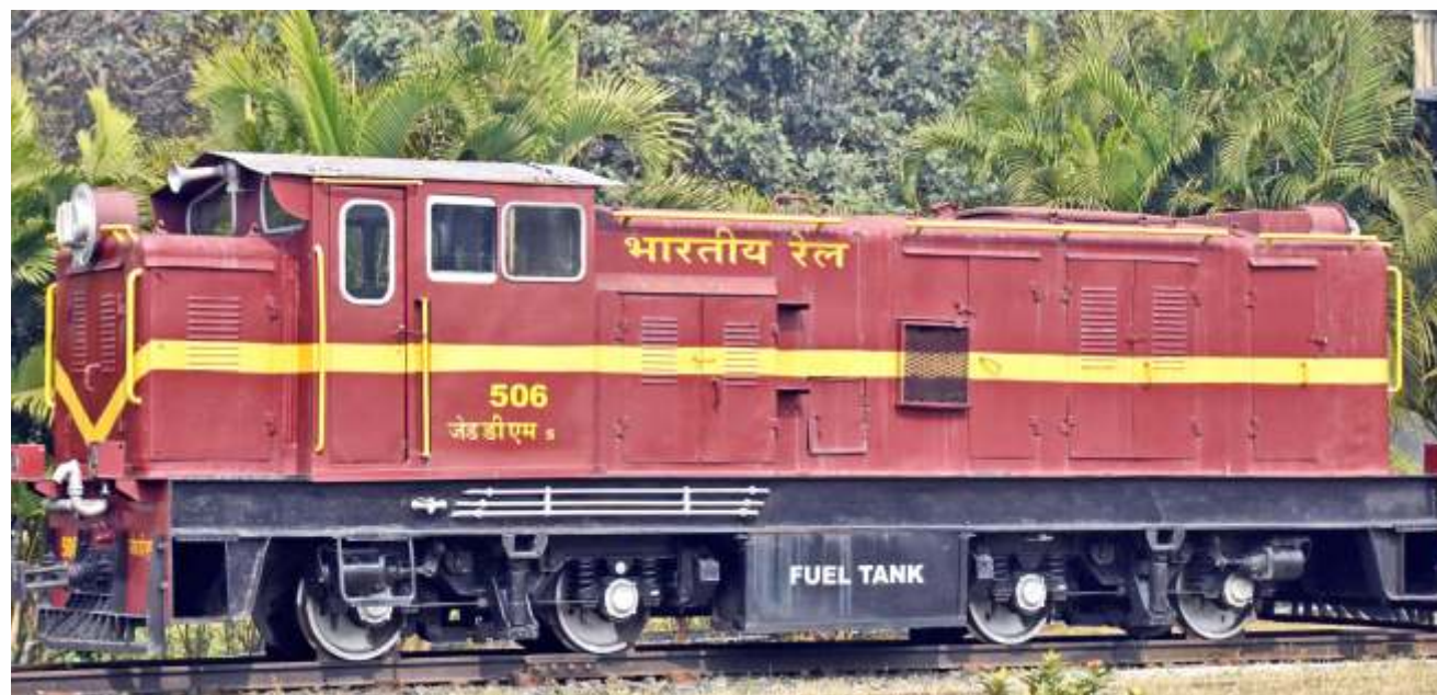
A Narrow Gauge diesel-hydraulic loco manufactured by CLW on display at the plant
