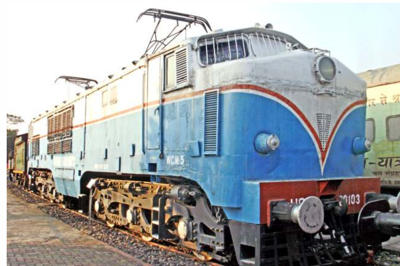
'Lokmanya', WCM5 class locomotive, the first 1500 V DC loco built by CLW. It can now be seen at the Rail Heritage Park at Howrah
